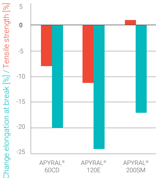
Figure 5: Change of the mechanical properties of the black EPDM compounds after ageing (100 °C, 7 days).
